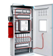
Electrical In-Cabinet Fire Suppression System
